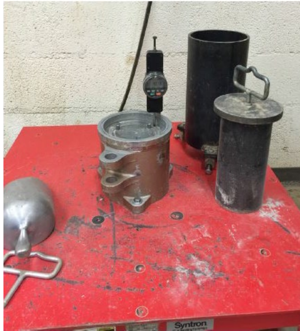
Figure 645K-34 Modified One Point Test for Drainfill Material
