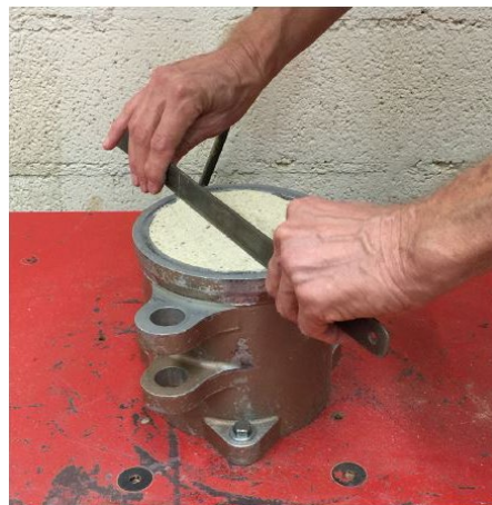
Figure 645K-32 Maximum Index Density is then determined by compacting the sand in the mold using a known weight and vibratory table (ASTM D4253). (NRCS – TX)
