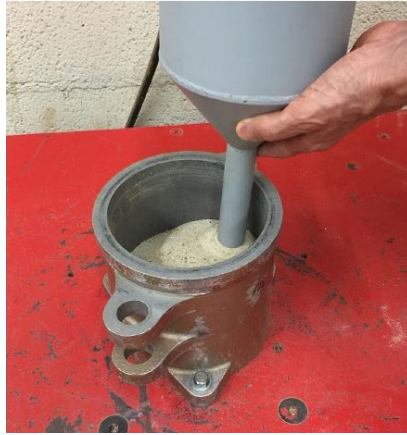
Figure 645K-31 Minimum Index Testing of Clean Sand. After filling the mold, screed off excess sand. Knowing the weight of the sand and the mold volume, the dry density is easily determined. (NRCS – TX)
