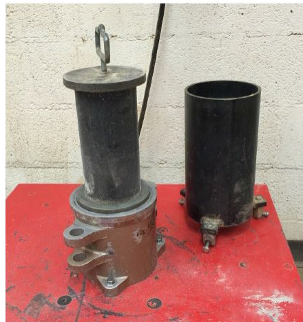
Figure 645K-32 Maximum Index Density is then determined by compacting the sand in the mold using a known weight and vibratory table (ASTM D4253). (NRCS – TX)
