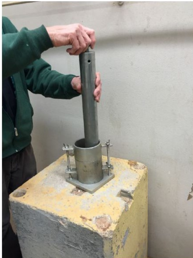
Figure 645K-34 Modified One Point Test for Drainfill Material
