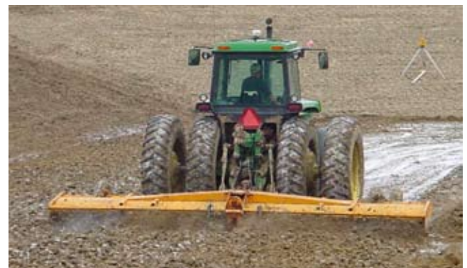
Figure 10D-23 High-speed rotary mixer used to mix dispersants into clays (Photo credit Jody Kraenzel, NRCS)
