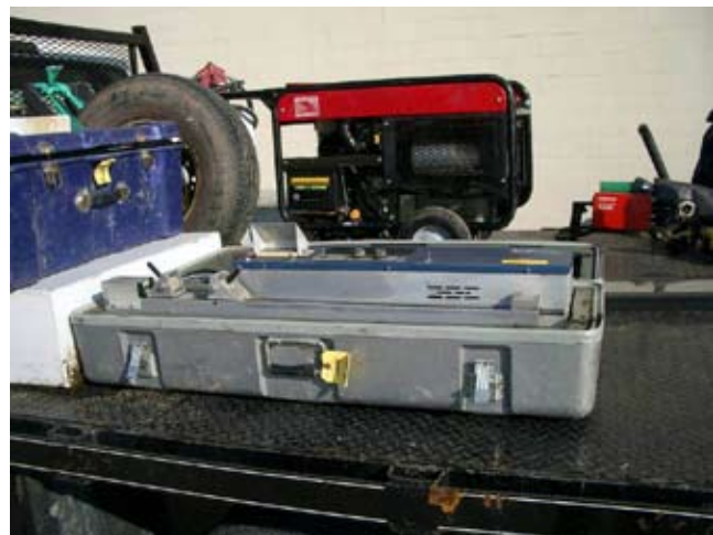
Figure 10E-22 Field tensiometer (Source: Poly-Flex, Inc., 1995)
