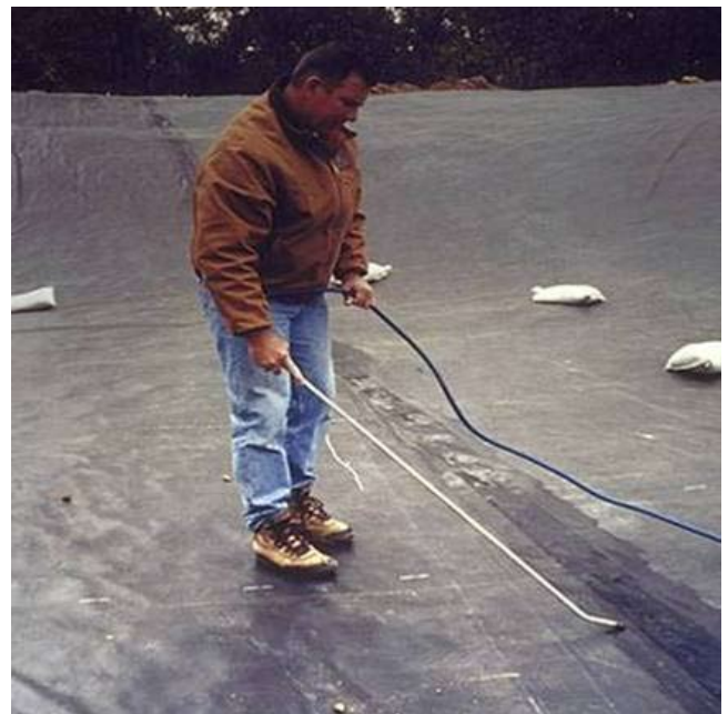
Figure 10E-19 Air lance test
