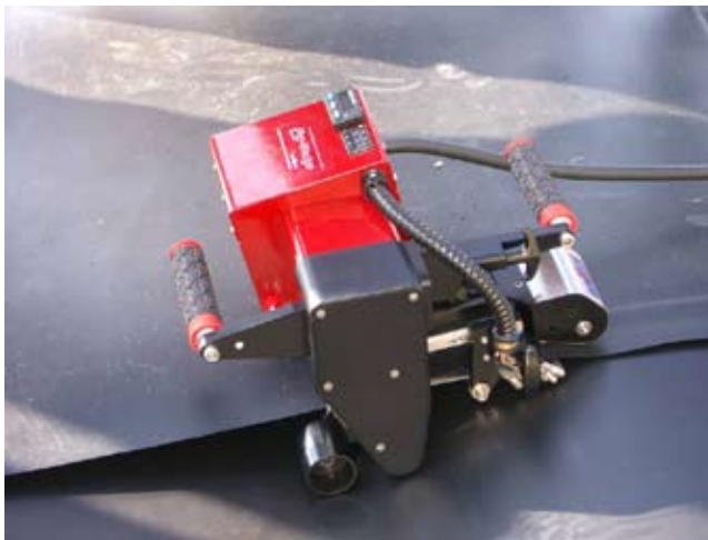
Figure 10E-14 Dual track hot wedge welder (Source: Poly-Flex, Inc., 1995)
