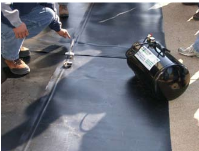
Figure 10E-18 Air channel test
