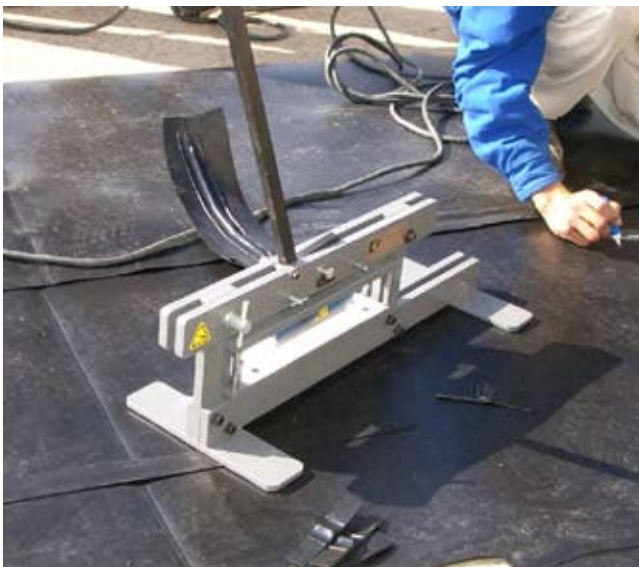
Figure 10E-21 Test specimen cutter
