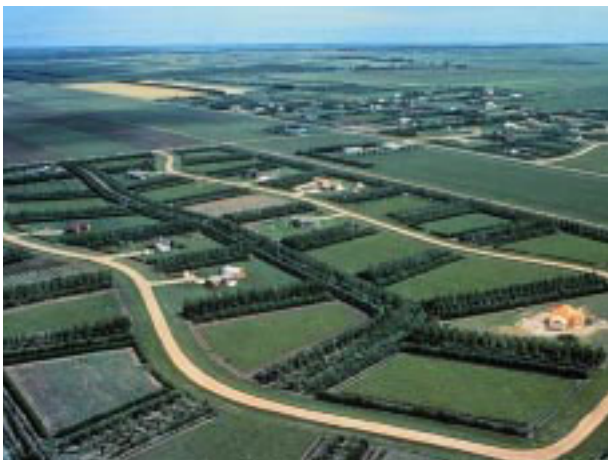
Figure 613–36 Windbreaks surrounding rural subdivision reduce energy consumption during the winter and lower snow removal costs (photo courtesy USDA NRCS)
