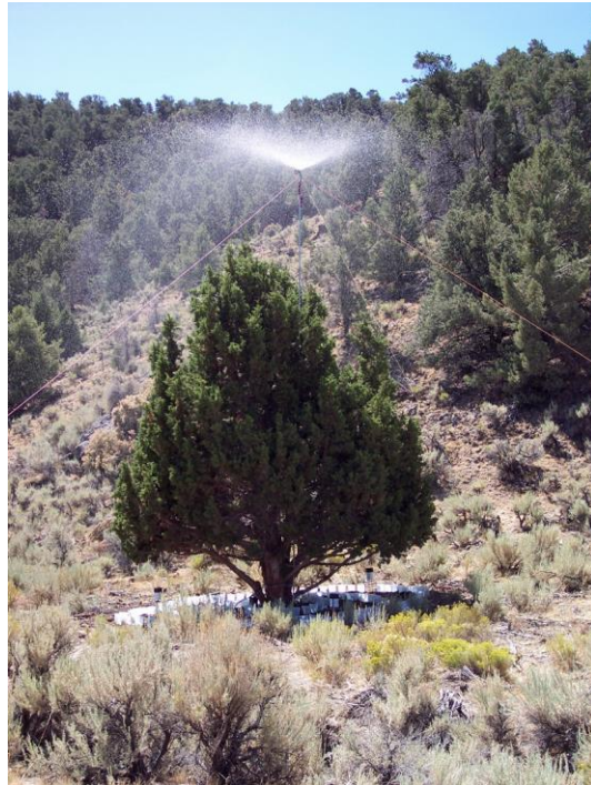
Figure A-10. Measuring interception, stemflow, and throughfall on a Juniper tree to determine components of the water balance on Wyoming Big sagebrush plant community that has been encroached by Juniper in Desatoya Mountains, central Nevada.
