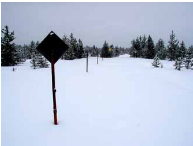
Figure 3–1 Snow courses—data are collected manually from multiple sample points along the snow course
