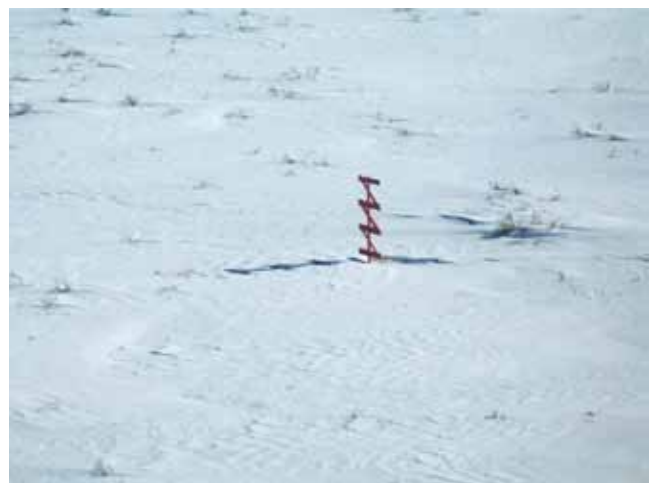
Figure 3–2 Aerial markers—data are observed manually from an aircraft because aerial markers are typically located in extremely remote locations with hazardous terrain
