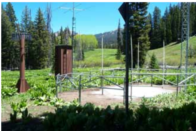
Figure 3–3 SNOTEL stations—snowpack and other hydrometeorological data are collected remotely and automatically transmitted to a central database
