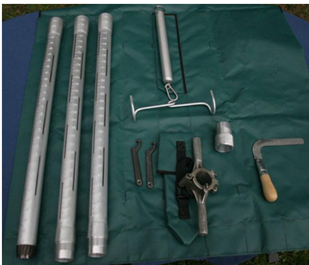
Figure 8B-1 Federal Snow Sampler set
