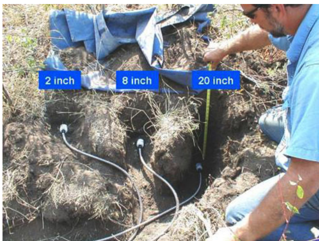
Figure 8C-1 Standard depths for sensing devices
