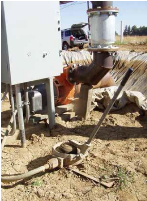
Figure 8–48 Diaphragm pump primer, tomato farm near Sacramento, CA
