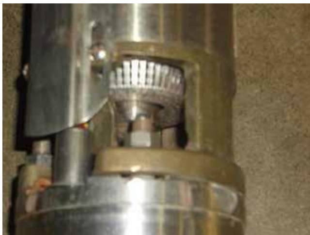
Figure 8–103 Submersible pump inlet screen
