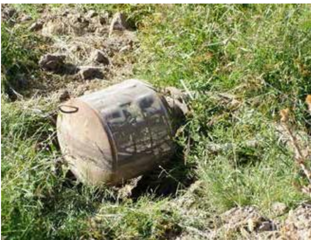
Figure 8–28 Example of pump intake screen cleaned by rotating sprays near Richland, WA
