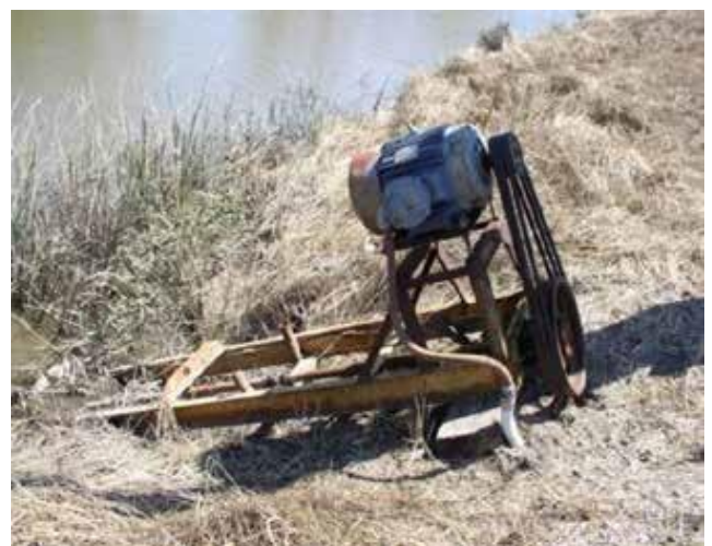
Figure 8–104 Propeller pump with unstable foundation near St. Martin, LA
