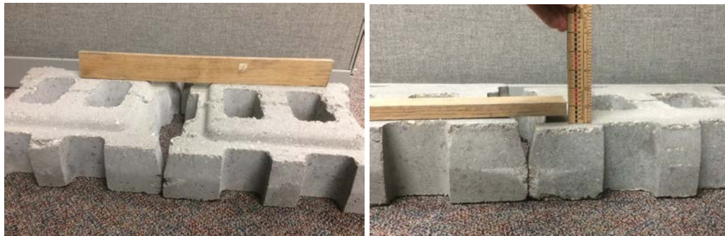
Figure 3: Untapered (Dome Top 2 ) ACB (left) and Flat-Top Tapered 3 ACB (right)
