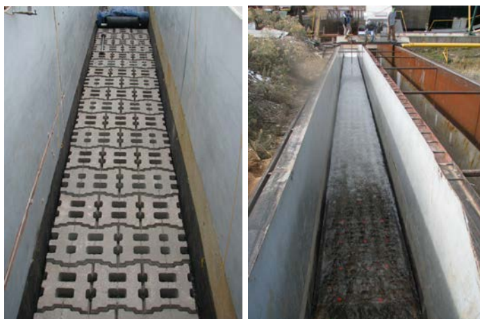
Figure 14: Flume Test for ACB at CSU Showing Placed ACBs (left) and Testing (right)
