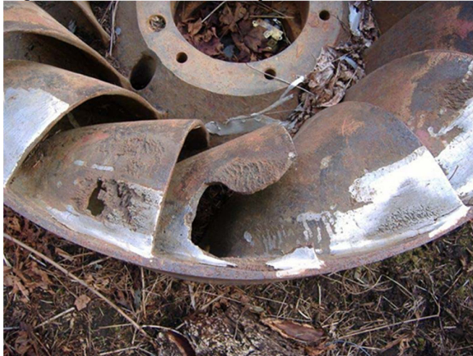
Figure 1-3: Cavitation Damage on the Propeller of a Francis Turbine
