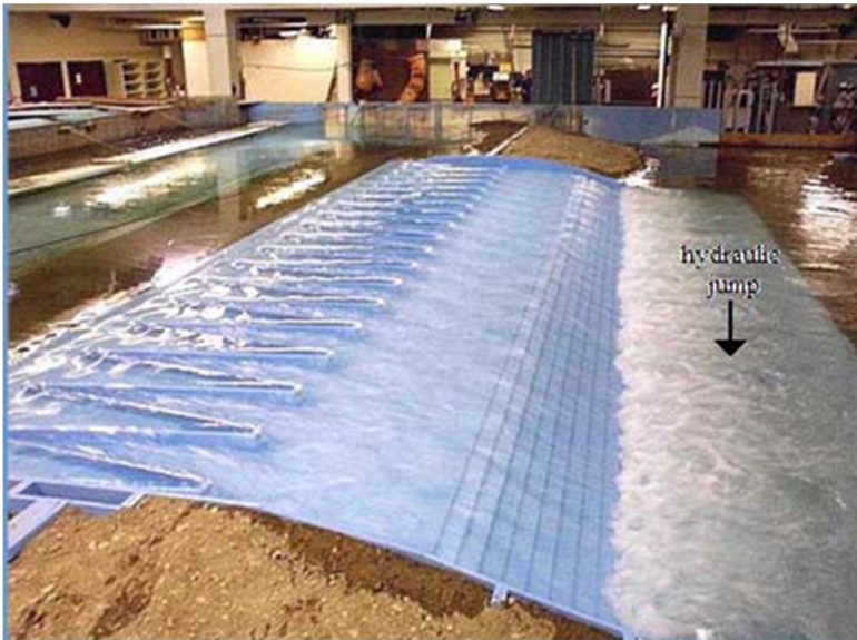
Figure 3-31: Hydraulic jump observed at the foot of a model spillway (courtesy of the Utah Water Research Laboratory).
