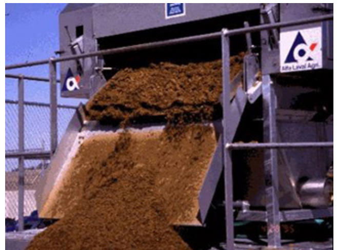
Figure 4–10 A rotating screen separator treating dairy manure (Iowa State University Cooperative Extension)
