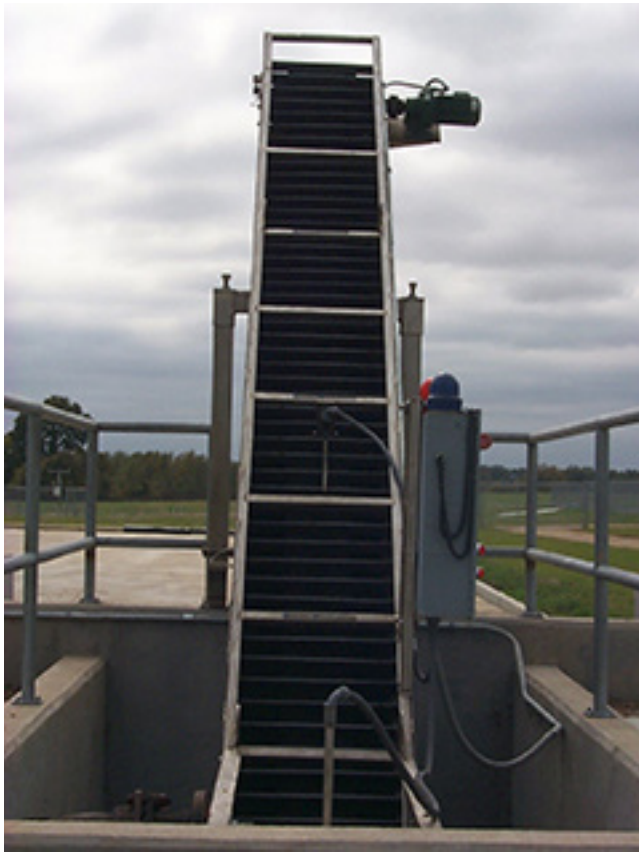
Figure 4–8 An in-channel flighted conveyor separator and solids stacking area (Mukhtar et al. 1999)
