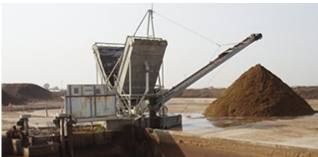
Figure 4–14 Solid-liquid separator that employs three techniques: fine stationary inclined screen (0.020 in), screw press, and an inclined flighted conveyor screen (courtesy of US FARM Systems, Tulare, CA)
