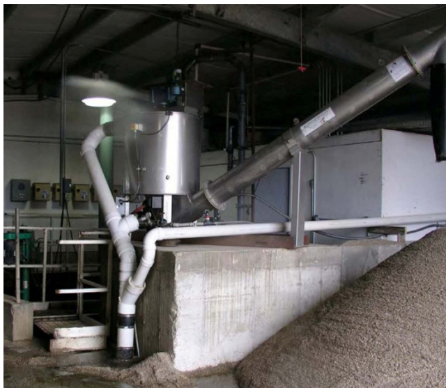
Figure 4-55 The Tru-Grit® Manure Sand Saver manufactured by Parkson Corporation (Holmes 2010)
