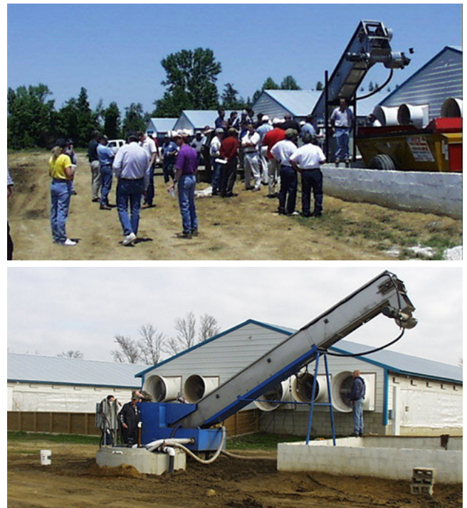
Figure 4–13 Combination of an in-channel flighted conveyor screen and a small screw press to treat liquid swine manure (Clemson University Extension)
