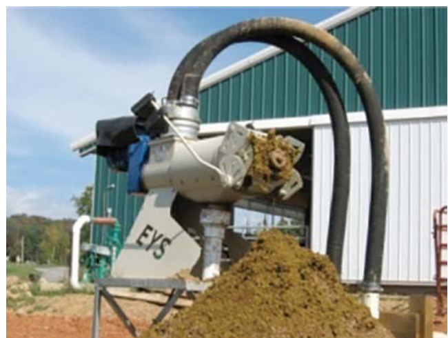
Figure 4–11 Two different designs of screw presses used to treat slurry manure (Virginia Polytechnic Institute, Virginia Cooperative Extension)
