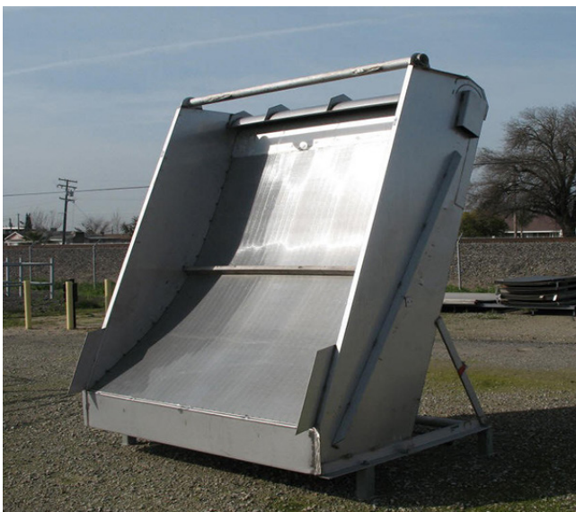
Figure 4-7 A stationary inclined bar screen and frame (courtesy of US FARM Systems, Tulare, CA)
