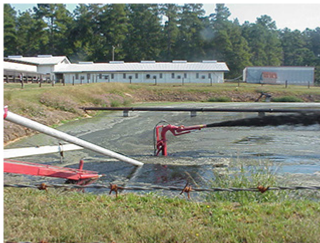
Figure 4–67 Agitation of a lagoon with a centrifugal chopper pump to remove sludge (Clemson University Cooperative Extension)
