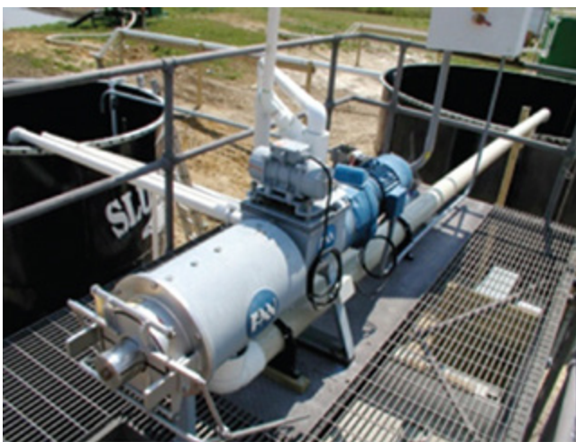
Figure 4–11 Two different designs of screw presses used to treat slurry manure (Virginia Polytechnic Institute, Virginia Cooperative Extension)
