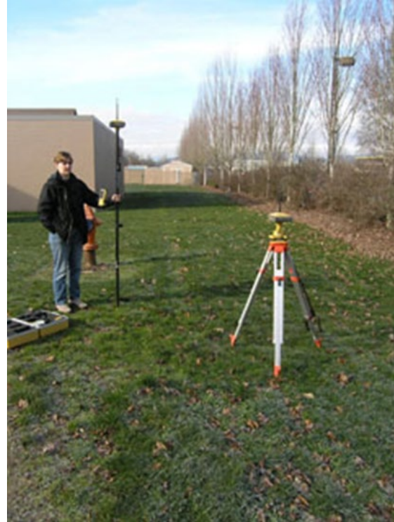
Figure 1-87: Typical setup for the base station over a known control point. The operator has used the optical plummet to center the base. Once the base is set, careful vertical measurement of the antenna slant height is made.
