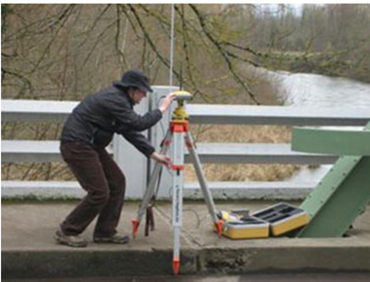
Figure 1-87: Typical setup for the base station over a known control point. The operator has used the optical plummet to center the base. Once the base is set, careful vertical measurement of the antenna slant height is made.
