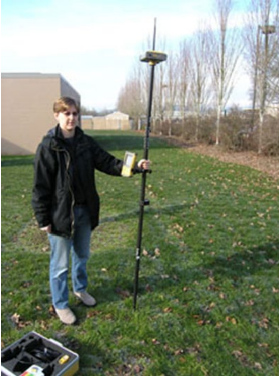
Figure 1-87: Typical setup for the base station over a known control point. The operator has used the optical plummet to center the base. Once the base is set, careful vertical measurement of the antenna slant height is made.
