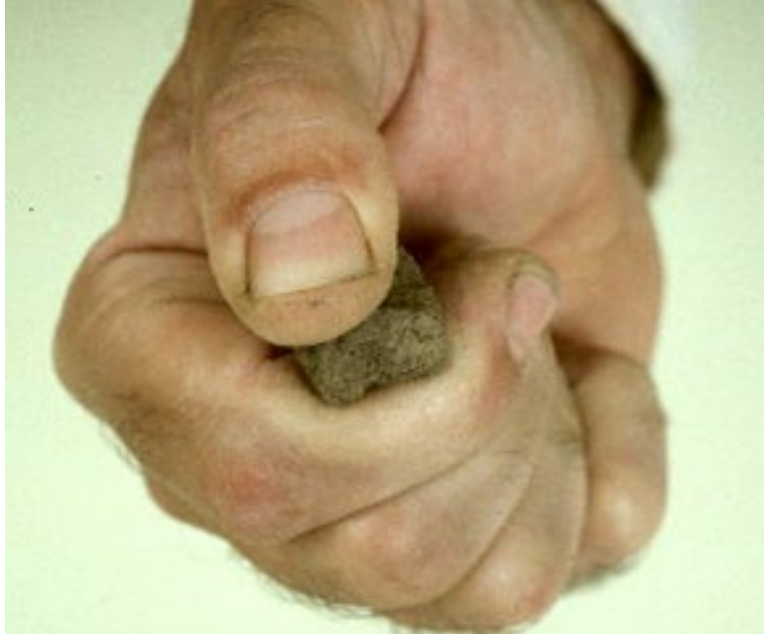
Figure 4-18: Crumbling a dried soil specimen to determine a soil's dry strength.
