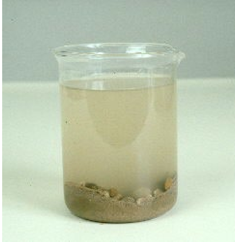
Figure 4-26: Estimating percentage of fines in a soil sample by dropping the sample in a beaker of water.
