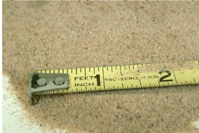
Figure 4-24: A poorly graded sample is predominately one size of particle.
