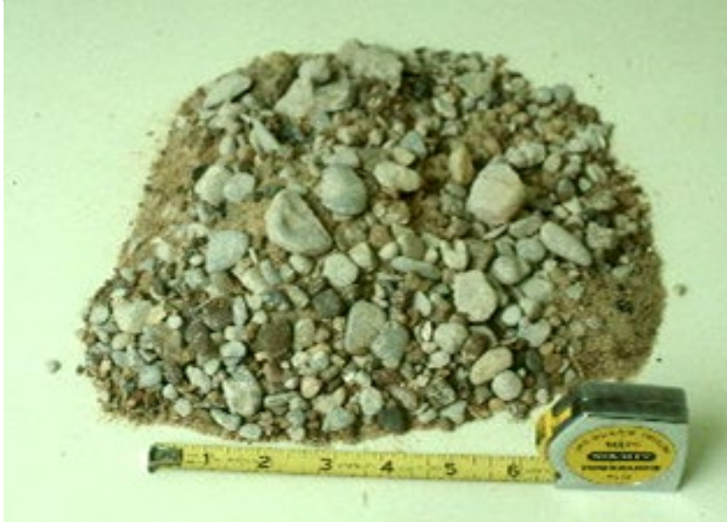
Figure 4-25: This Photograph represents a WELL graded sample has a wide range of particle sizes that are about equally distributed by weight.
