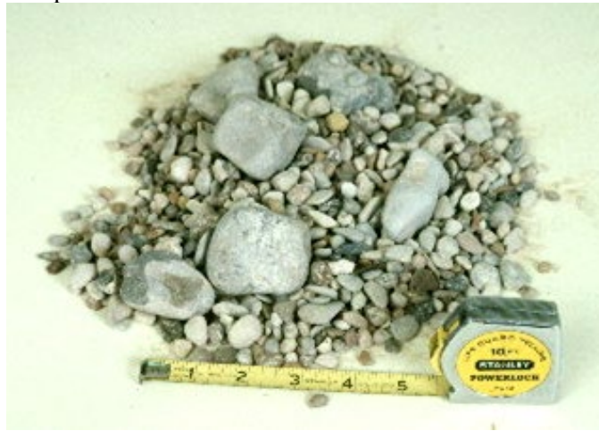
Figure 4-23: This Photograph represents a POOR (gap/uniformed)-graded sample has a range of particle sizes missing. This sample has coarse and fine but no medium size particles.
