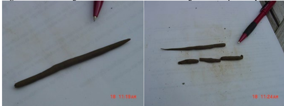
Figure 4-17: Rolling threads to determine a soil's toughness and plasticity.
