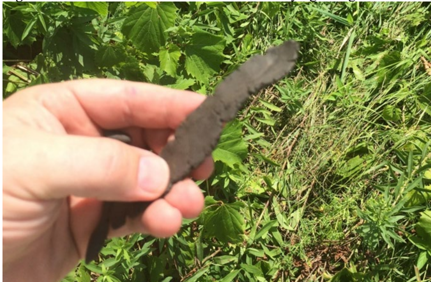
Figure 4-21: The ribbon test is useful for classifying fine-grained soils.
