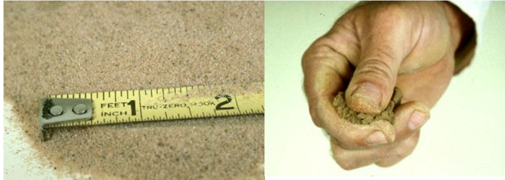
Figure 4-16: Visual and manual techniques are important tools for classifying soils in the field.
