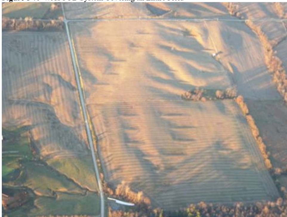
Figure 8-7: WASCOB System Covering an Entire Field
