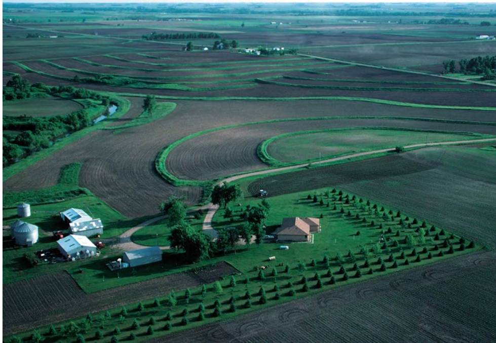
Figure 8-29: Terraces with Parallel Alignment
