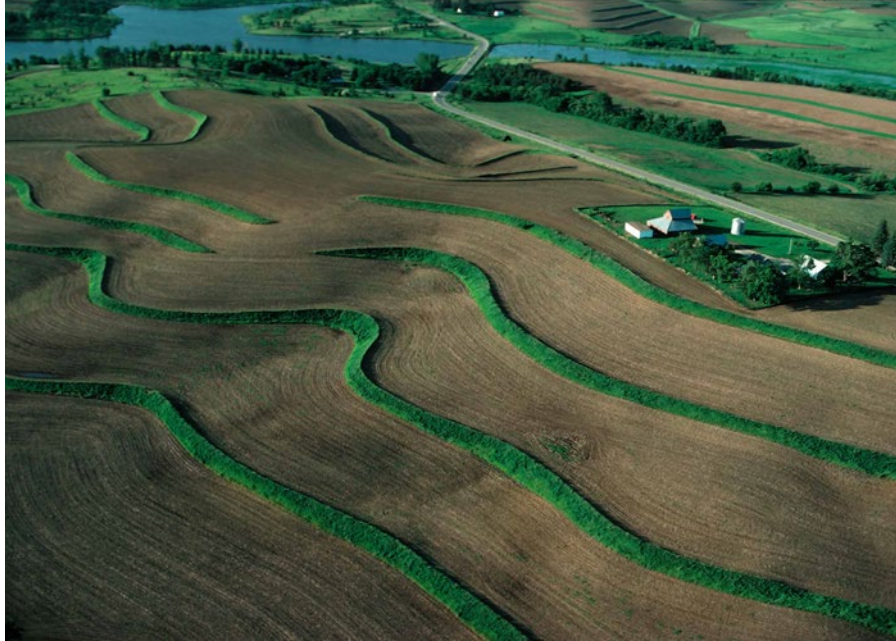
Figure 8-3: Steep-back Terraces Controlling Gully Erosion
