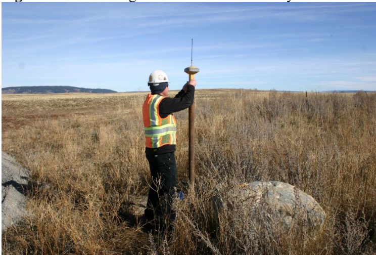
Figure 11-20: Setting a Benchmark with Survey Grade GPS
