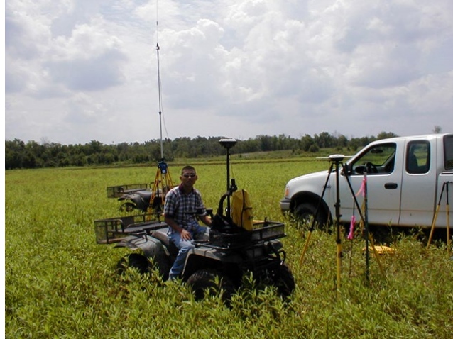
Figure 13-17: Survey-grade GPS equipment increases the efficiency of topographic surveys.
