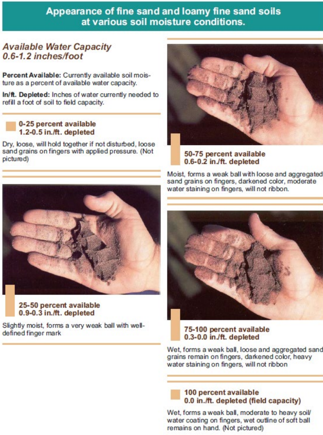
Figure 15-8: Appearance of Soils at Various Soil Moisture Conditions
