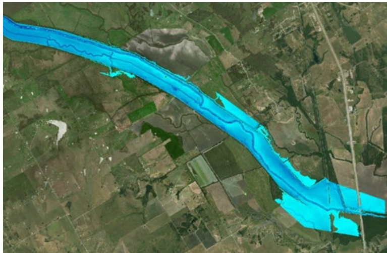
Figure 19-43: Example Use of HEC-RAS in Two Dimensions to Examine a RIVERINE Wetland
