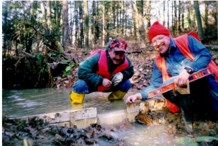
Figure 19-35: Flow Measurement Using a Sharp-Crested Weir
