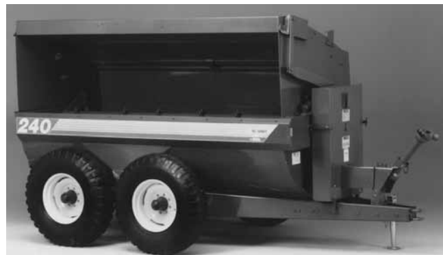
Figure 12–99 Flail-type side unload spreader (Bartok 1994) (Photo courtesy of Ideal Industries, Inc.)
