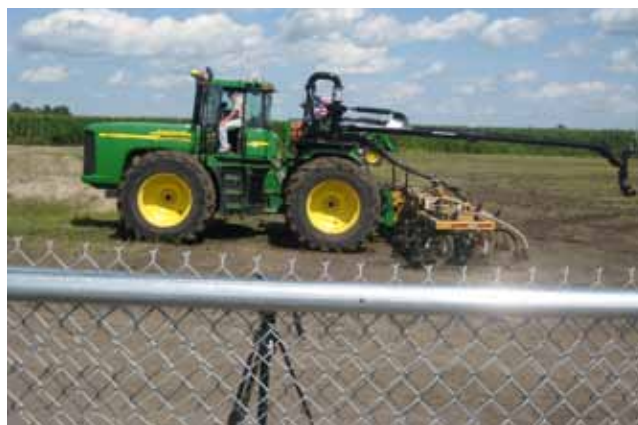
Figure 12–116 Hose reels for supply line and drag hose (Photos by Bill Boyd, NRCS)
