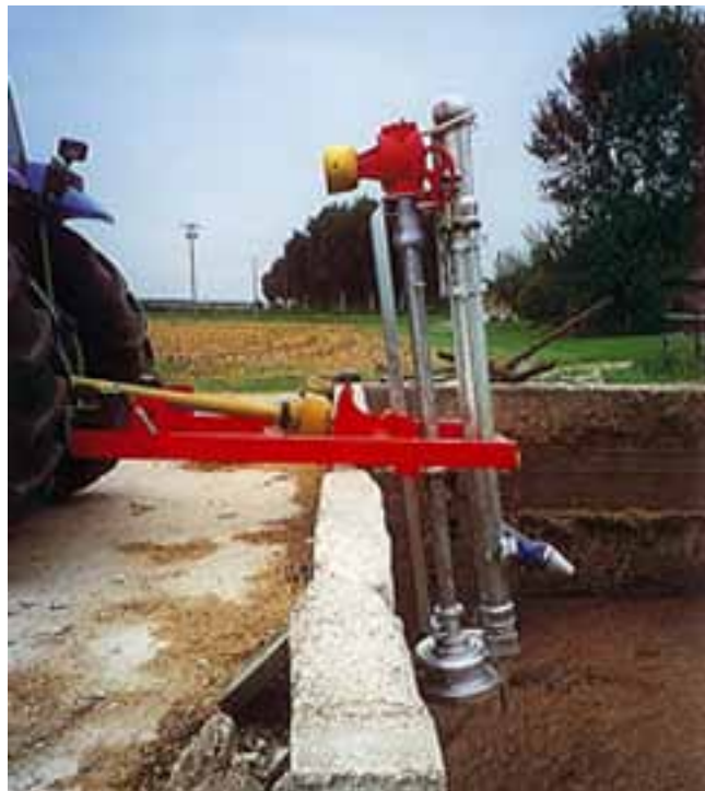
Figure 12-54 Vertical shaft PTO-powered chopper-agitator pump (Photo courtesy of DODA U.S.A., Inc.)
