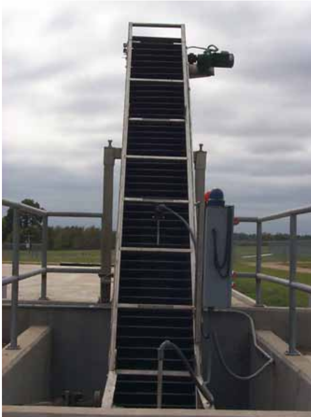
Figure 12-74 Pump and pipeline loaded conveyor separator (Photo and drawing courtesy of Albers Manure Handling Systems, Inc.)
