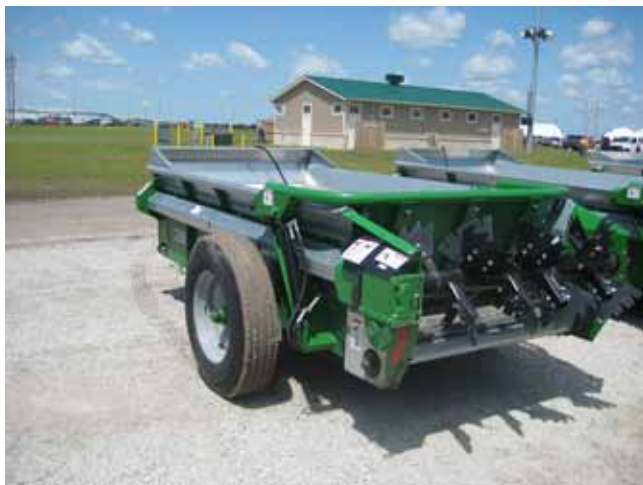
Figure 12-94 Cross bar conveyor box spreader (Reprinted with permission of New Holland Agriculture)
