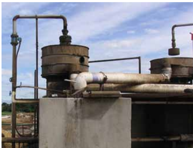
Figure 12-77 Vibrating screen separator (Photo by Dave Moffitt, retired, NRCS)
