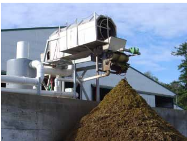
Figure 12-76 Rotating screen coupled with roller press (Photo courtesy of Accent Mfg.)
