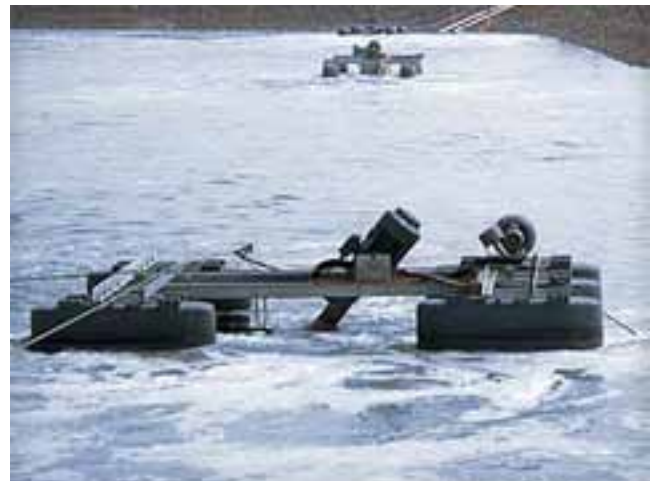
Figure 12-63 Floating aerators for liquid waste aeration ( Drawing and photo courtesy of Aeromix Systems, Inc., and Patrick Charles Pty Ltd. )
