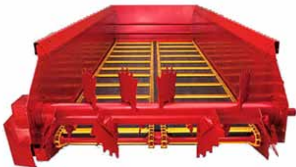
Figure 12-94 Cross bar conveyor box spreader (Reprinted with permission of New Holland Agriculture)
