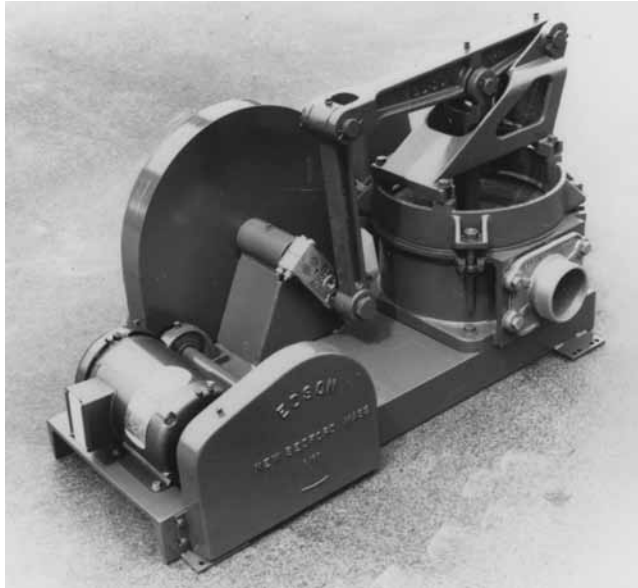
Figure 12-37 Diaphragm pump (Photo and drawing courtesy of Protek Specialty Co.)
