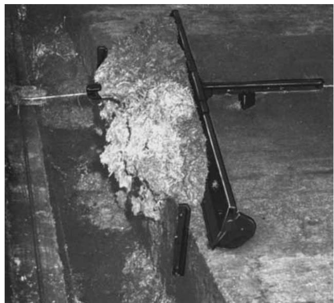
Figure 12–20 Cable-drive scraper for open alley or under slat floor ( Photo courtesy of Acorn Equipment Co. )
