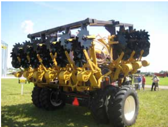
Figure 12–112 Disc-type manure injector used to minimize soil disturbance folded for transport (Photo by Bill Boyd, NRCS)
