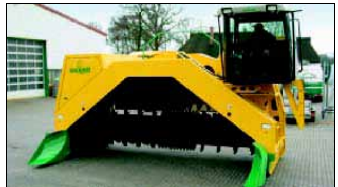
Figure 12–60 Self-propelled compost turners ( Photo courtesy of Backhus )
