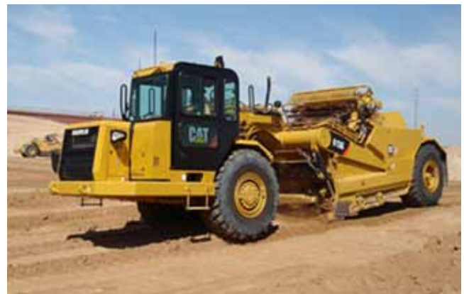
Figure 12–19 Self-propelled, self-loading elevating scraper-hauler (Photo courtesy of Caterpillar®)
