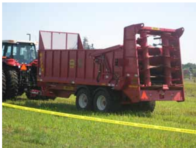
Figure 12–96 Box spreader with vertical-mounted beaters (Photo by Bill Boyd, NRCS)
