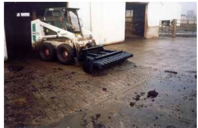
Figure 12-10 Rubber tire scraper blade/diamond groove concrete (Photo courtesy of Mensch Mfg.)
