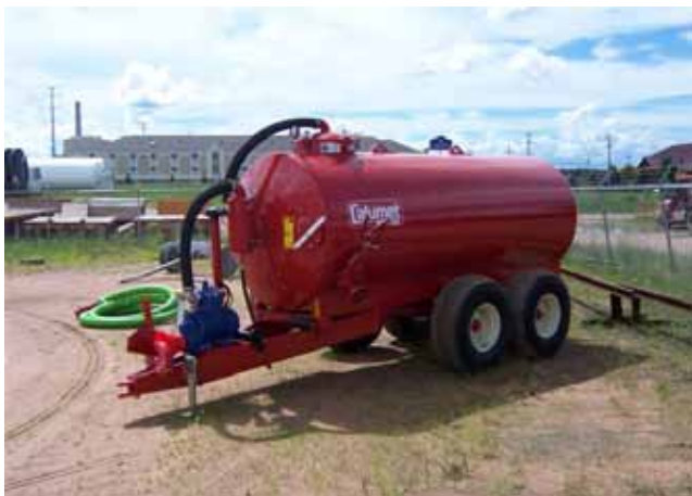
Figure 12–104 Vacuum tank spreader (Photo courtesy of Calumet)
