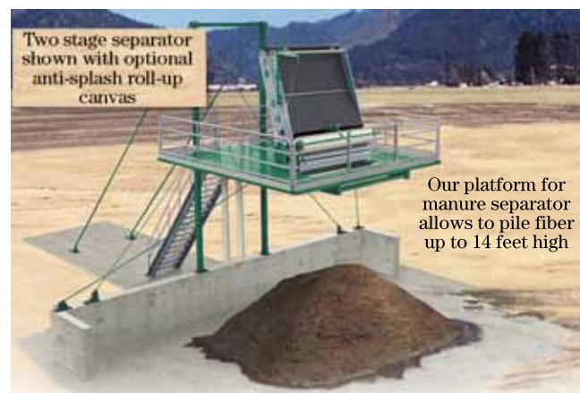
Figure 12-72 Static inclined screen separator with incorporated press roller ( Photo courtesy of CADY, Inc. )
