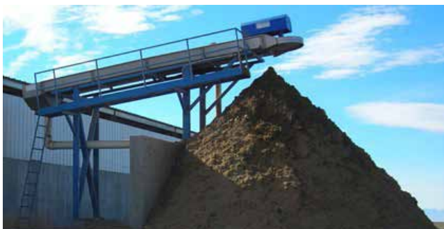
Figure 12-74 Pump and pipeline loaded conveyor separator (Photo and drawing courtesy of Albers Manure Handling Systems, Inc.)
