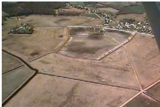
Figure 2-7 Channelized stream (lower left); former natural stream has been assimilated into the regional artificial drainage network
