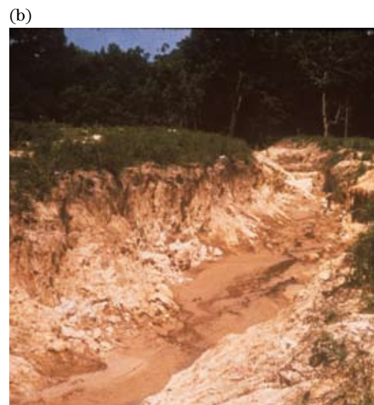
Figure TS14A–24 Photographs of exposure of dispersive clays in streamside slopes in TX and OK
