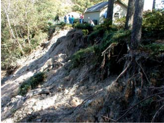
Figure TS14A-4 Failed streambank in Tarboro, NC, following high channel flows following Hurricane Floyd. Erosion of the toe caused bank instability in the slope. Measures to protect the toe of the slope are essential, in addition to assuring stability of the system.
