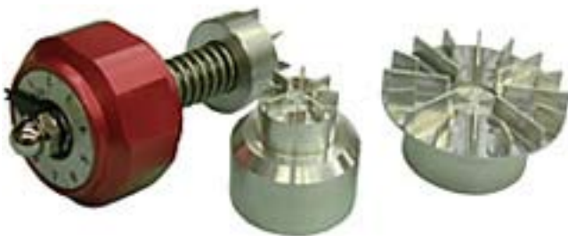
Figure TS14A-1 Hand held torvane device ( Photo courtesy Geotest Instruments, Inc. )
