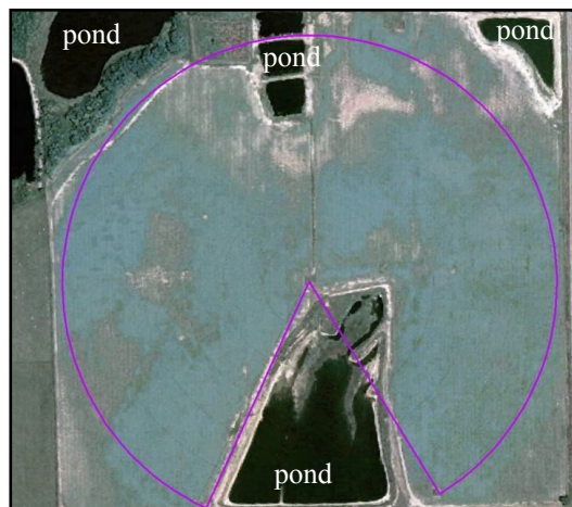
Figure SC6-50 Although ideally suited and operate most efficiently in circular or rectangular fields, they can be fitted to complex field situations, especially if fitted with a VRI system.
