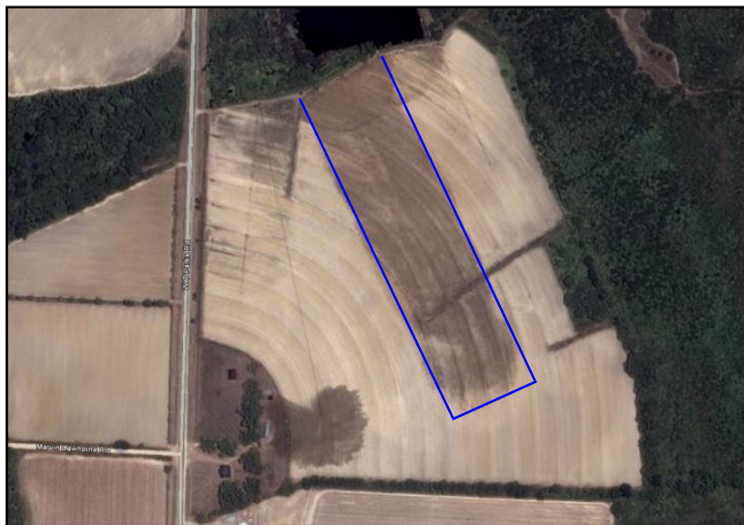
Figure SC6-47 Typical wetted pattern of one application run with a traveler (big gun) system
