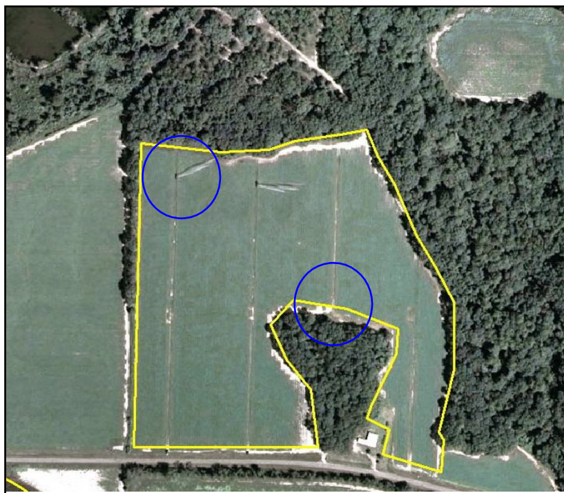
Figure SC6-48 Ideally, fields used with traveler systems are rectangular with a water supply main and row of riser connections through the center providing application overlap. Odd shaped fields can also be irrigated effectively with modifications for travel run times and a little tolerance for overlap.
