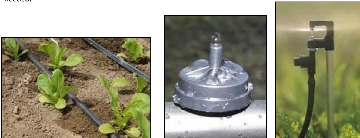
Figure SC6-37 Lateral (drip) tape (left), drip emitter (center) and microsprayer (right) device
