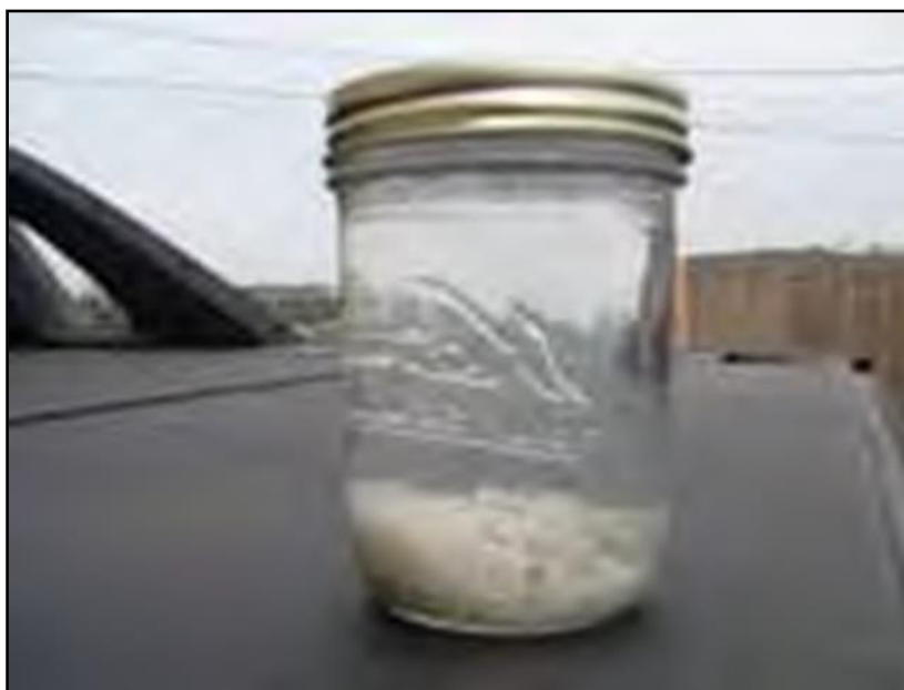
Figure SC6-38 Precipitate indicates reaction between fertilizer/chemical and water that will clog drip tape or emitters
