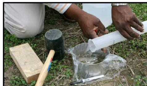
Figure 7: Preparing soil infiltration test
