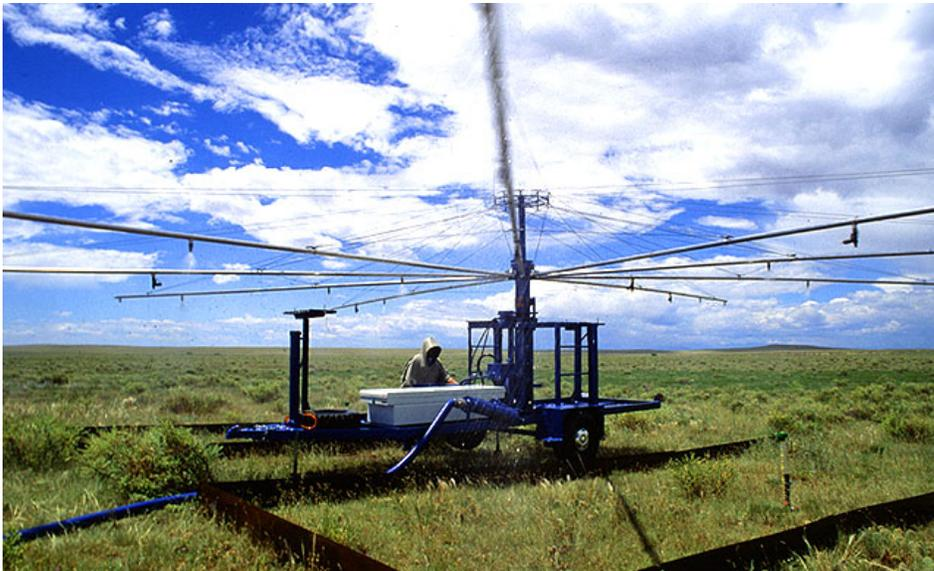
**Figure D-7.** Walnut Gulch rainfall simulator used to collect data near Moab, Utah for development of the Rangeland Hydrology and Erosion Model (RHEM). Plots were 2m (6ft) wide by 6m (20ft) long.
