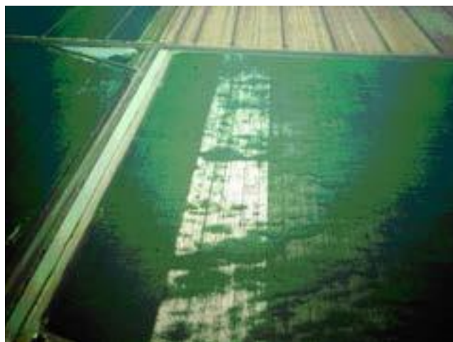
Figure 7–10 Matured cotton field, showing the difference in crop uniformity between the SDI-irrigated field (left-hand side of photo) next to a furrow-irrigated field (middle and right-hand side of photo) (courtesy C.J. Phene USDA-ARS)
