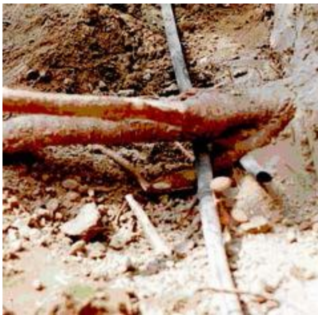
Figure 7–13 An example of a root pinching the SDI lateral (cut lateral on the right) in a pistachio orchard with the SDI lateral installed 5 feet (1.52 m) from the tree row and 18 to 20 inches (0.46–0.51 m) deep
