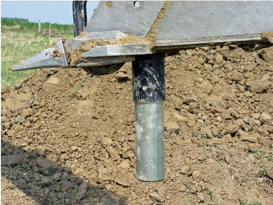
Figure 5-9. Shelby tube sampler mounted to a backhoe bucket.
