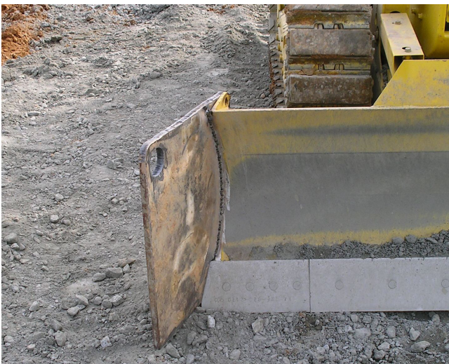
Figure 13–11 Dozer blade retrofitted with sides
