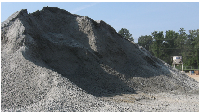
Figure 13–2 Materials that fall from the upper portion of a steep pile will segregate
