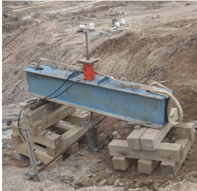
Figure 645R-31. Micropile Tensile Load Test (NRCS-OK)
